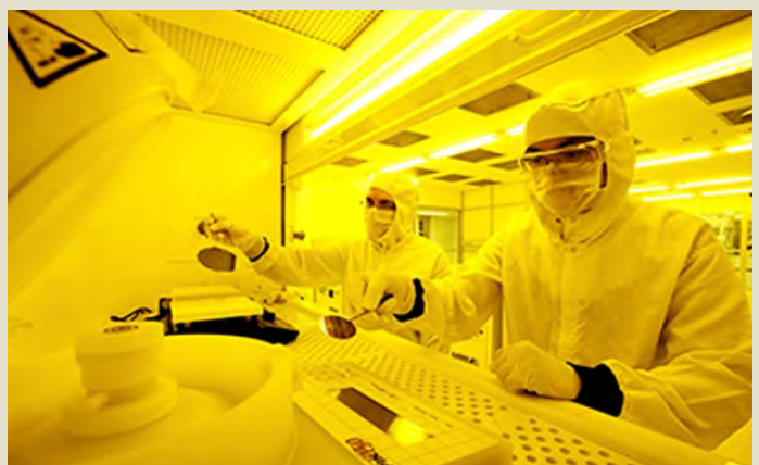
Figure 1 Researchers performing resist coating in a class 10 semiconductor nanofabrication cleanroom.
