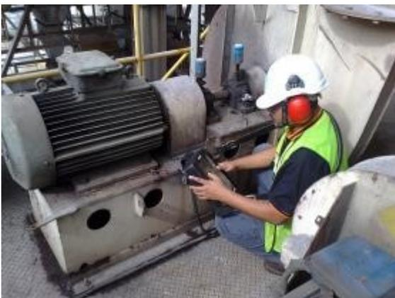
Figure 1: Vibration analysis of motor & fan impeller at Shah Alam, Malaysia
