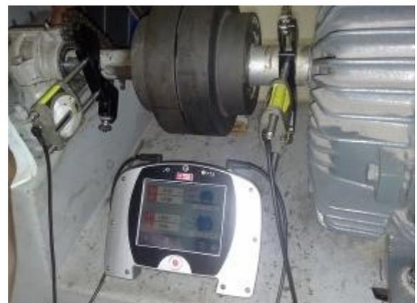
Figure 3: Laser alignment shaft to shaft
