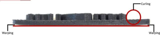
Figure 2: Illustration of 3D printed parts with the warp and curl defects.
