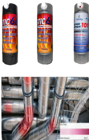
Figure 5: Smart Thermal Indicating Coating with an irreversible color change above 60°C as active visual inspection to detect wet Insulation/damaged insulation.
